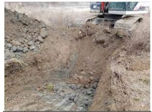
Photo Further example view of test pitting of stockpiled soils (1/6/2021). Note debris, gravel and spoils in soils.
