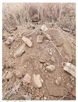
Photo 2 – Excavated fill at Test Pit TP-2.
